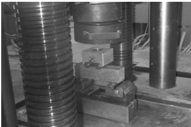
Figure 2 Flexural strength test.
